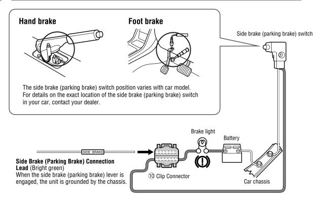
Attach a Clip Connector 10 to the end of the side brake (parking brake) connection lead.
